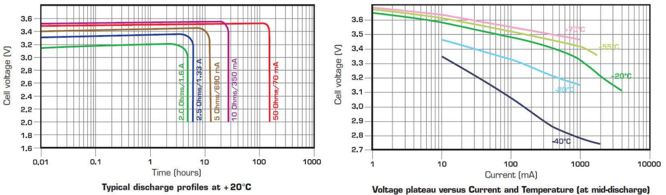
Fig. 1 - LSH 20 primary lithium battery graphs
