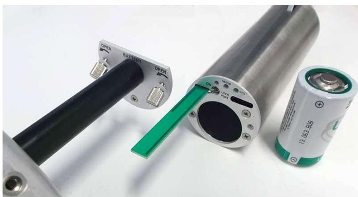
Extensive, sporadic current consumption during the modem transmission phases makes it even more difficult to evaluate battery status. This is due to voltage changes consequent to internal thermal and chemical variations induced by the current peaks.
